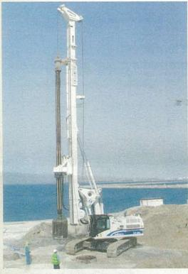
ith the new SR-80 C, Soilmec has reached its target to complete a range of drilling rigs for large-diameter piles and remarkable depths.
