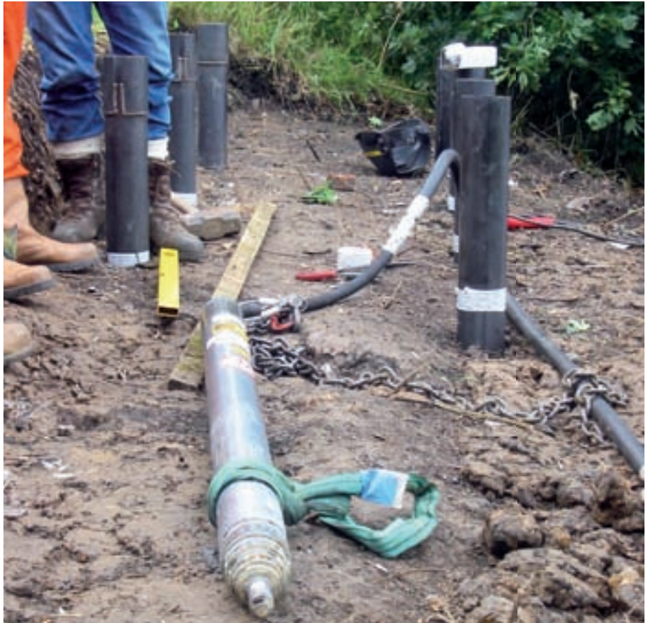
Tracto Technik's Grundomat soil-displacement hammer
