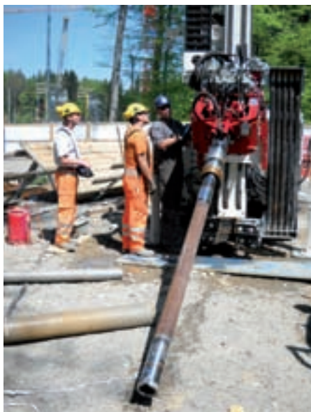
SonicSampDrill CRS-V crawler rig with tilting head
