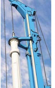
can be transported complete with kelly bar hence reducing the site installation times. Thanks to the new Soilmec concept design, the SR-45 shows very good performances in traditional bored piles with kelly bars – but also in cased piles - and it can be easily reconfigured to perform different drilling technologies such as continuous flight au-
