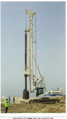
drilling rig for LDP and CFA. After the great success earned by the SR-70, SR-90, and SR-100 introduced since 2005, Soilmec offers to the demanding foundation market the possibility to choose a new rig combining in the same machine the experience of SR Soilmec series and that of Caterpillar. In fact SR-80 C is a perfect mix of CAT base machine turret (345 C) with Soilmec standard rotary.
