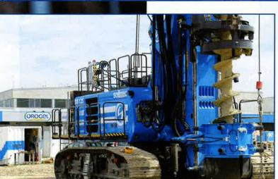
Orogel industrial plants in Cesena (486 piles), was made precisely by the drilling rig Sollmec SR-125 HIT in CFA configuration (continuous flight auger) technology. The SR-125 HIT (High Technology) is the first Soilmec machine equipped with new Brigade Electronics safety devices (five Elite cameras and Smart bbs-tek acoustic advice).
