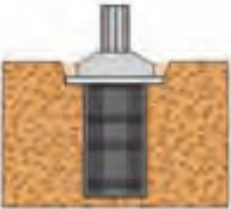
Foundation elements Barrettes
