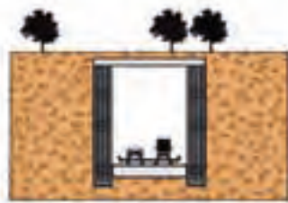
Reinforced DW Permanent foundation walls
